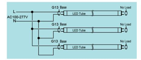
• Fourth Step: Affix the field applied label to the light fixture. Then install the tube. The tube is single port wiring connection.
