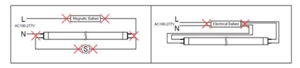
• Third Step: Install the LED tube and make the electrical connection
